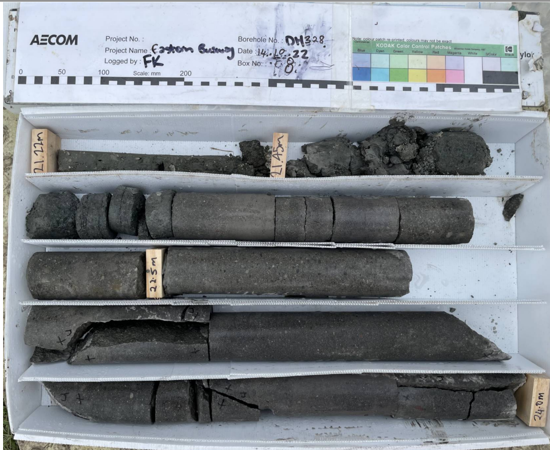
Box: 8 of 10 - Depth: P\DH328_P 21.22m to 24.0m of 28.50m Date Drilled 13/10/2022 to 14/10/2022 - Date Photographed: 14/10/2022
