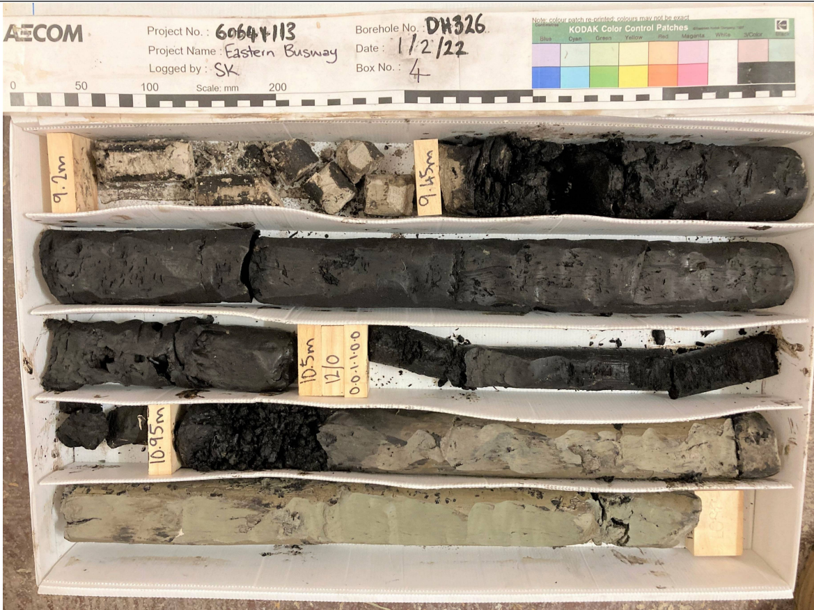
Box: 4 of 9 - Depth: 09.20m to 12.00m of 24.78m Date Drilled 1/02/2022 to 2/02/2022 - Date Photographed: 1/02/2022
