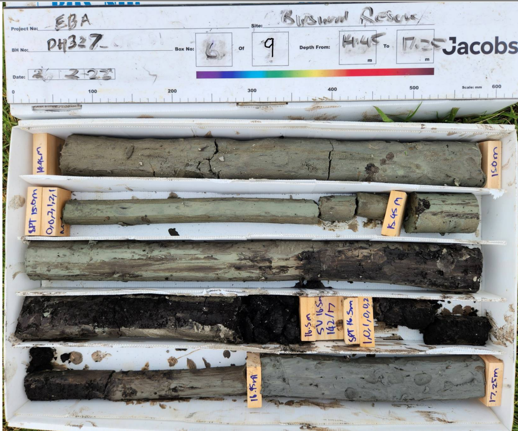
Box: 6 of 9 - Depth: 14.45m to 17.25m of 25.50m Date Drilled 2/02/2023 to 2/02/2023 - Date Photographed: 2/02/2023
