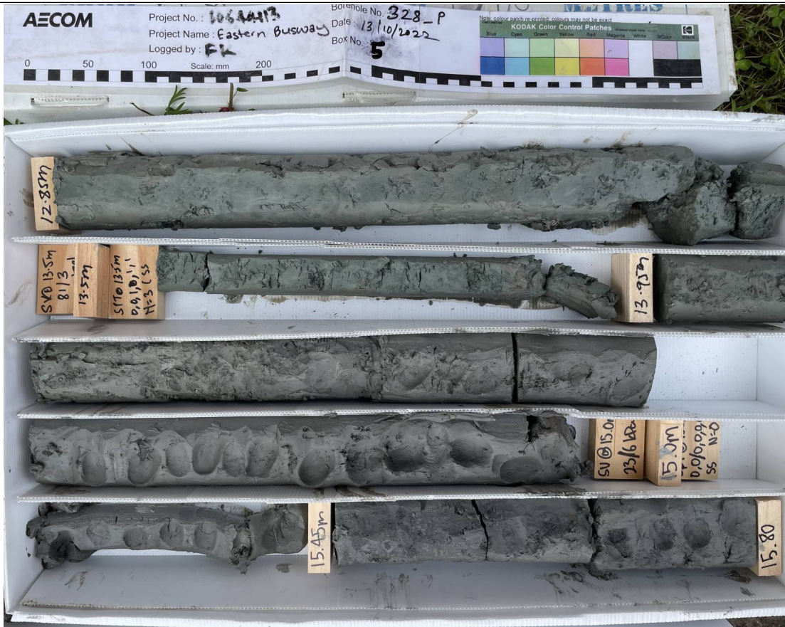
Box: 5 of 10 - Depth: P\DH328_P 12.85m to 15.80m of 28.50m Date Drilled 13/10/2022 to 14/10/2022 - Date Photographed: 13/10/2022
